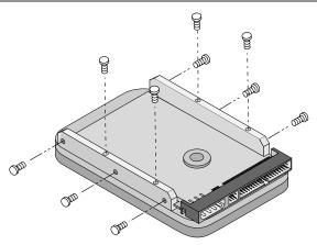
3 Slide the drive carefully into the drive bay. Secure the drive with four 6-32 UNC mounting screws in either the sidemounting holes or the bottom-mounting holes. Do not overtighten the screws. Do not use metric screws or screws more than 1/4 inch long for mounting the drive.
